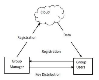
Figure 2. Dynamic Broadcast Encryption.
